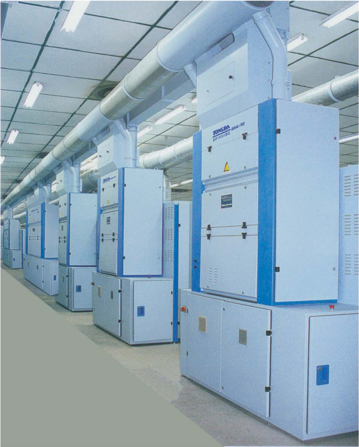
This machine is a connecting unit between cards and blowroom whose function is to make fiber (after being opened and mixed) feed to card in even butt ensure continuous and even cotton Supply for card.
